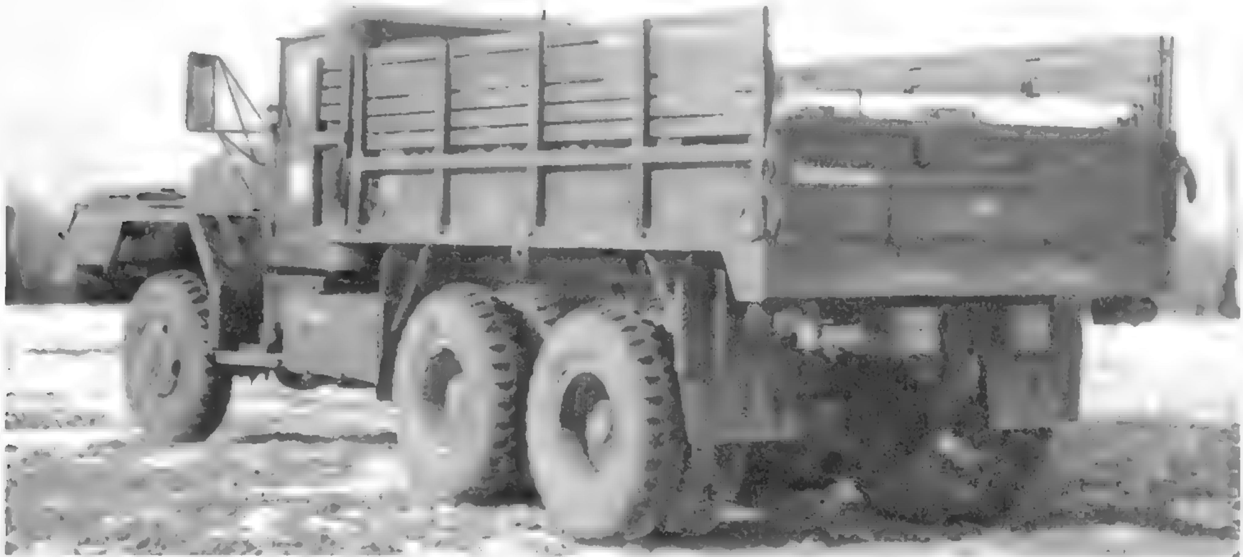
The center portion of the sideboards of the M54A1, like the M54 and M41, folded down to form troop seats. (Photo courtesy of the Patton Museum)
